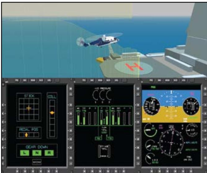
The Sikorsky S-92 is equipped with a Multi Purpose Flight Data Recorder (MPFR), which collects data from all aircraft instruments onboard. This information is downloaded on a daily basis by Cougar Avionics, and is then processed in FlightScape software. Standard Operation Procedures, or SOP filters have been configured in FlightScape and are run
